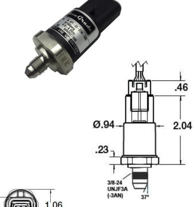
\*\*\*Warning: Applying torque to the plastic sensor body will damage the unit which will void any return privileges. Do NOT hold the sensor by the body when tightening the fluid connection. Only use the stainless steel wrench hex to tighten the fluid connection to the sensor.
